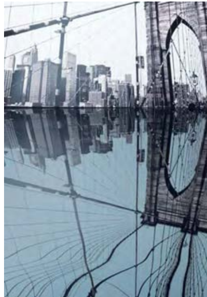
Industry Typical Tempered Glass roll-wave of .008
