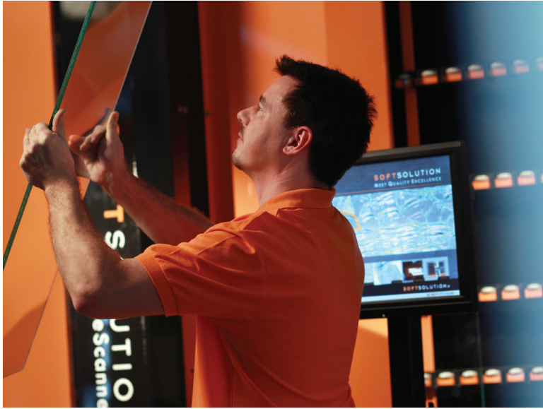
Left: Scanning and quality-control equipment, like the SoftSolution LineScanner, detect glass defects, helping to keep bad glass from getting to customers and stopping companies from adding any more value into the glass if it is already defective. A modified version of the pictured scanner is sold in North America through Fenetech as the FeneVision LineScanner. Above: A glass edge chip detected by a scanner.
